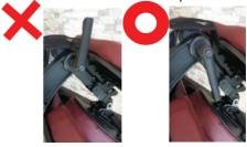
7. Loosen headrest height adjustment knob and headrest cam lever
